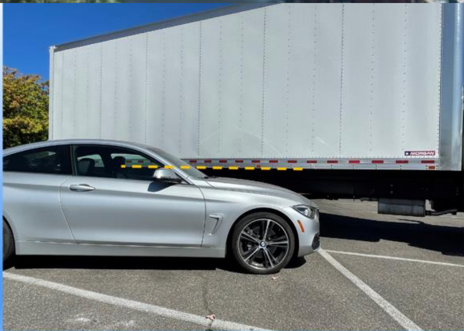
Underride happens with Single Unit Trucks as well as tractor trailers.
