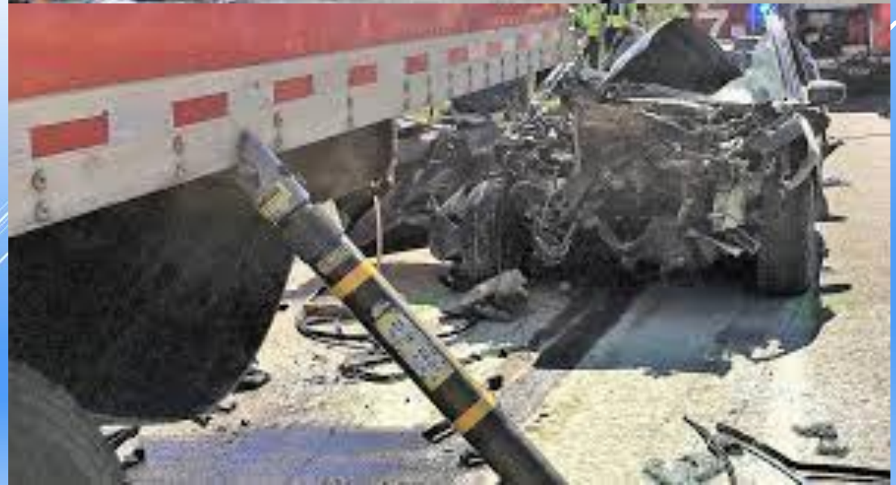
Underride happens with Single Unit Trucks as well as tractor trailers.
